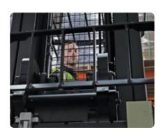
NOTCHED LOAD BACKREST WITH ANGLED BAR ☼ — helps provide operators with natural sight lines for clear view when picking up and dropping off pallets
