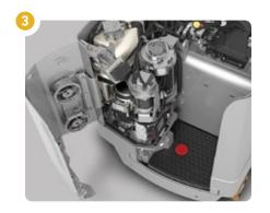
ACCESS DOOR AND COVERS provide technicians tool-free access to motors and controls.
