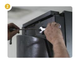
MAST WEAR PLUGS allow for mast adjustments in just 15 minutes - no shims, gauges or disassembly required
