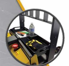
The MPB-VG with standard battery pack includes an operator convenience tray with large storage area. Units equipped with a 9" battery box have several convenience tray options. (9" battery box option shown.)
